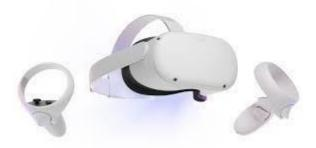
**11.** Haptic Devices: Haptic devices are input and output devices that provide users with a tactile or force feedback response. They are commonly used in gaming and virtual reality applications.
