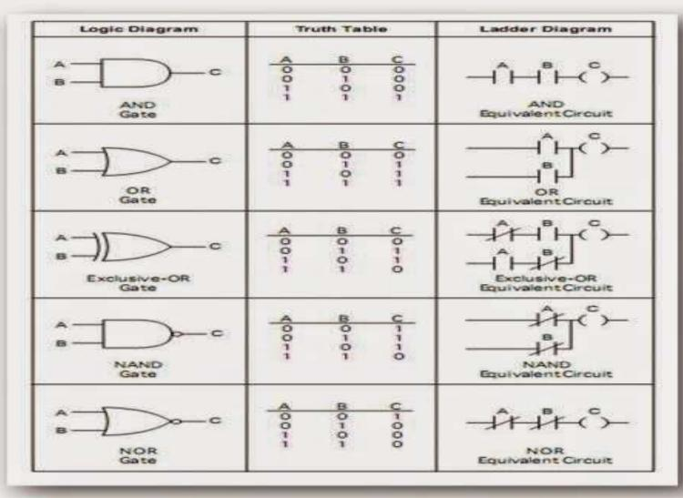
**OR Combination:** For logical 'OR' combination of two or more inputs are put in parallel to each other. The rung condition will be TRUE if any one of the input is true if the inputs are false then only the rung condition will be false.
