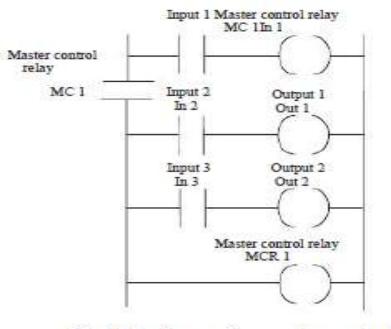
Principle of use of a master control relay.
